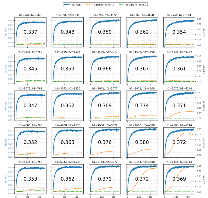
Fig. 5: Validation accuracy and \hat{\rho} trends for a 2-layer MLP with varying hidden unit configurations (h_1, h_2) on CIFAR100, optimized via grid search.
