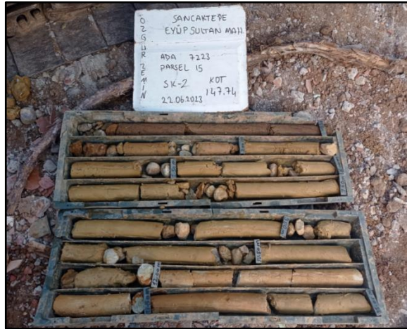
Figure 5.5 Soil core samples obtained from Borehole SK-2
