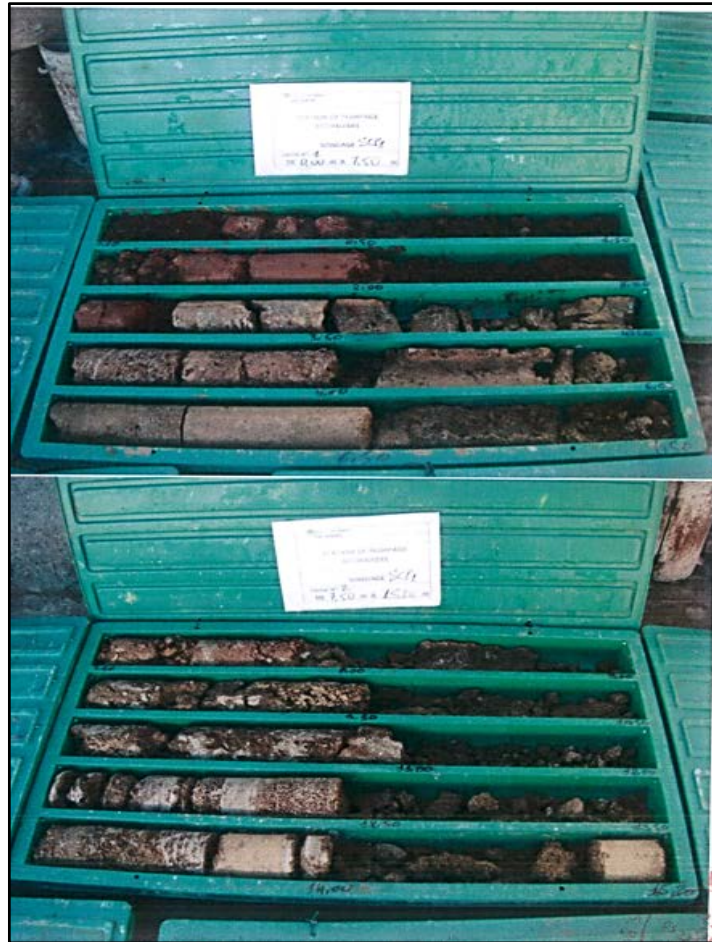
Figure 5.11 Sample Box Display Of Borehole SCP1 Investigation
