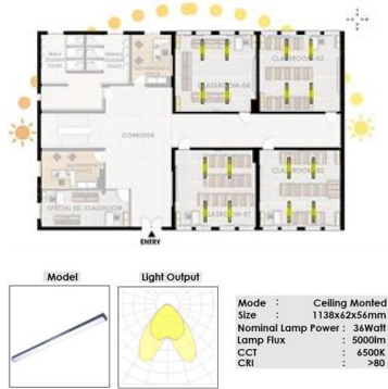
Figure 3. The electrical lighting fixture used in the classrooms is LED fixtures
