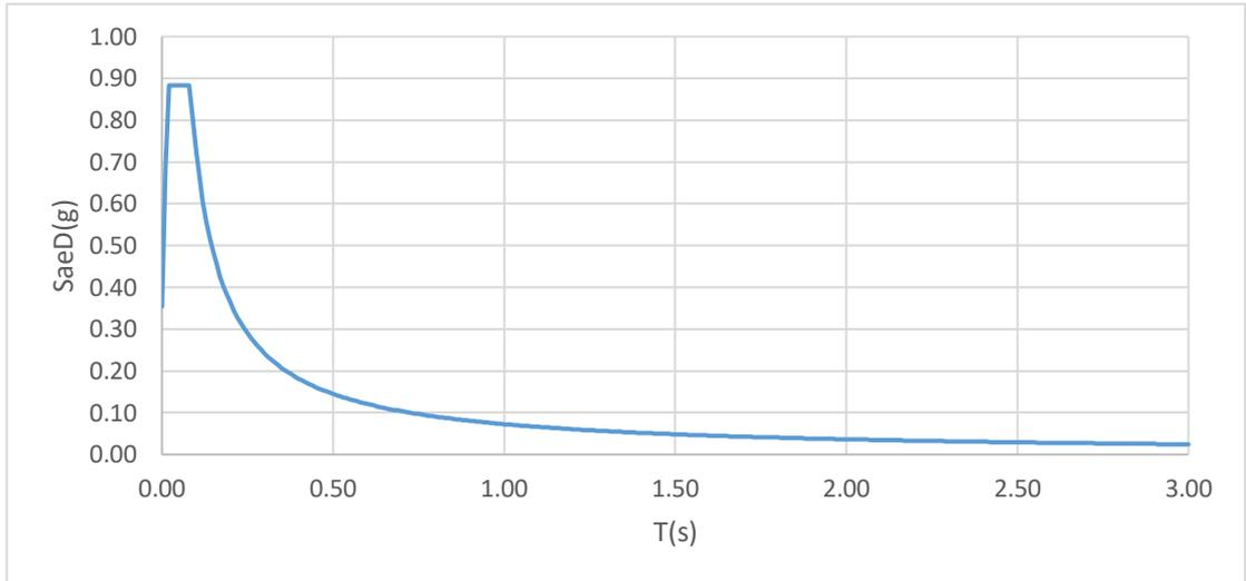
**Figure 4.49** DD-1 earthquake level vertical elastic design acceleration spectrum
