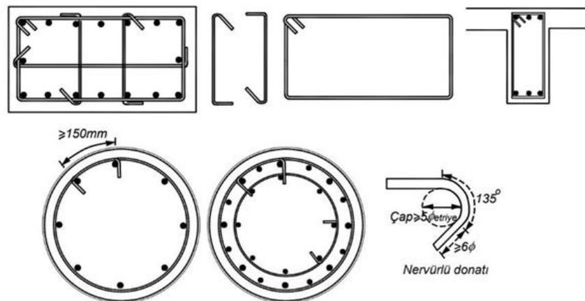
**Figure 3.7** Special earthquake stirrups and cross-ties (Celep, 2017).
