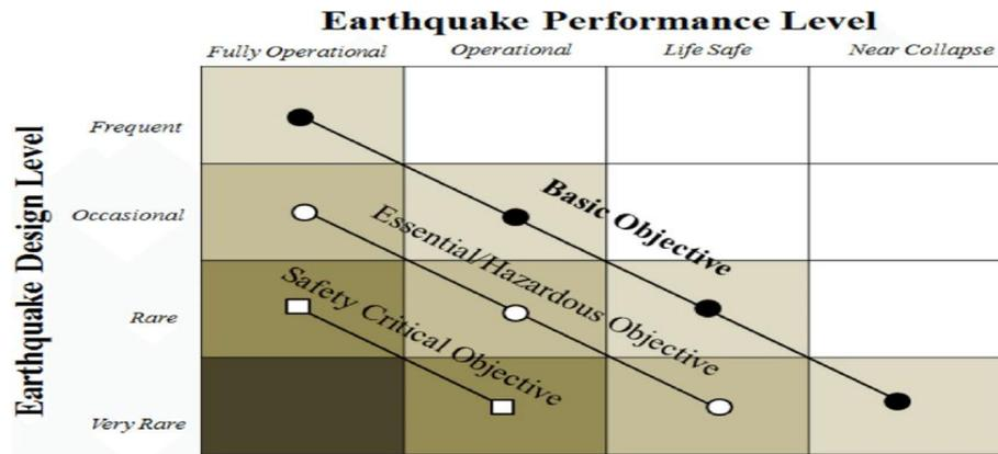
**Figure 2.2** Performance Objectives for buildings (Leelataviwat et al., 1999).
