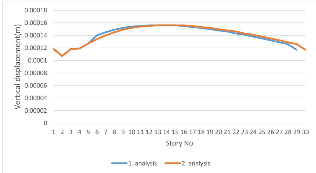
**Figure 4.4** Creep calculation of vertical story displacements.
