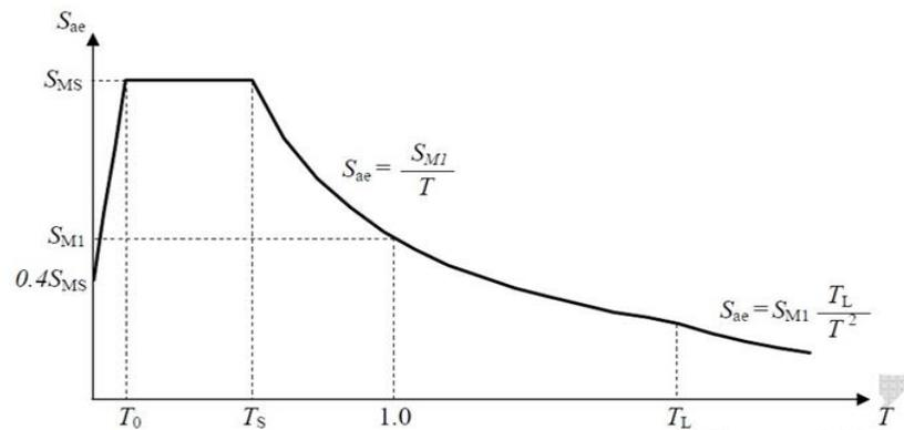
**Figure 2.4** Elastic design spectrum curve according to IYBDY.
