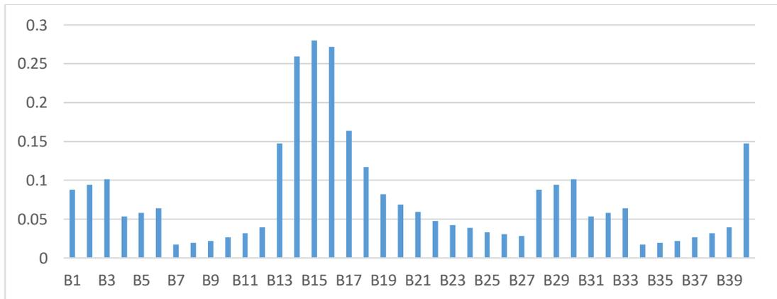
**Figure 4.23** Shear force D/C ratios of 11th floor beams.
