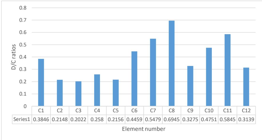
**Figure 4.38** 20th floor column P-M-M D/C ratios.
