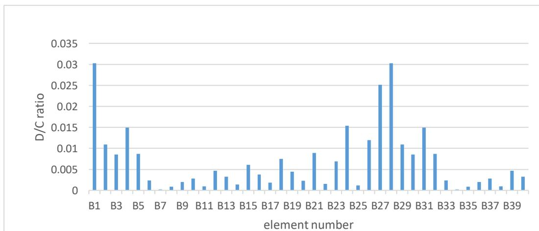
**Figure 4.26** Moment D/C ratios of 1<sup>st</sup> story beams.
