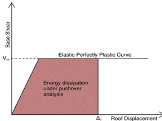
**Figure 3.4** Push-over curve of elastic displacement.
