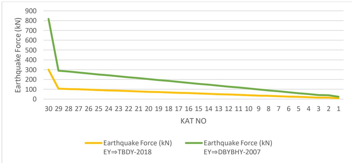
**Figure 4.41** Comparison of 2007 and 2018 Y Direction Seismic Forces.
