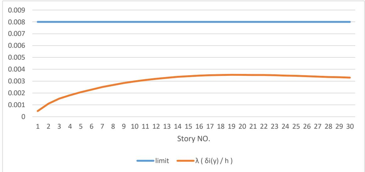
**Figure 4.11** Relative story drifts in Y-Y directions.
