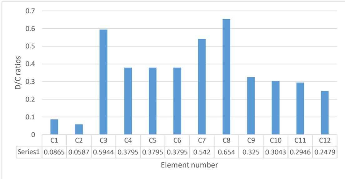
**Figure 4.34** 20th story column shear force D/C ratios.
