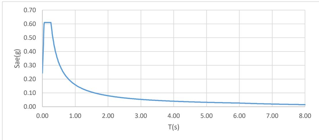
**Figure 4.48** DD-1 earthquake level horizontal elastic design acceleration spectrum.
