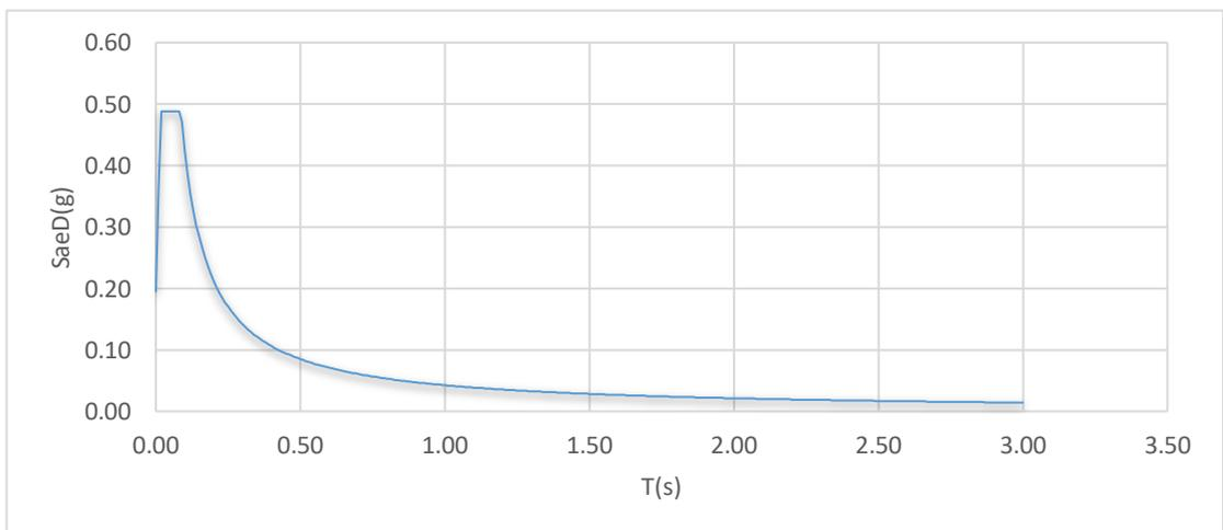
**Figure 4.18** DD-4 earthquake level vertical elastic design acceleration spectrum.
