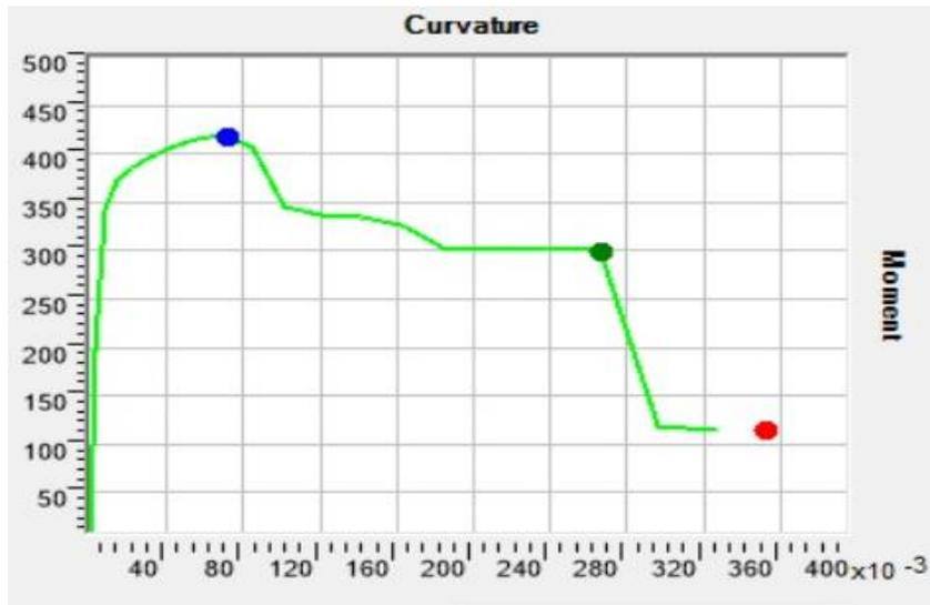
**Figure 4.19** 50/80 beam moment capacity curve.
