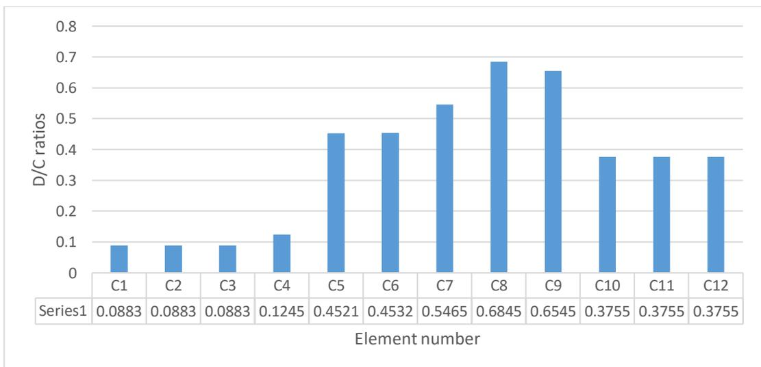
**Figure 4.33** 11th floor column shear force D/C ratios
