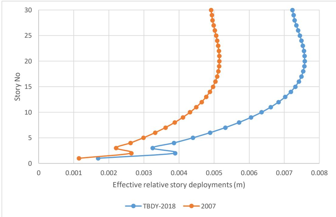
**Figure 4.45** Comparison of y-direction-enabled relative story offsets
