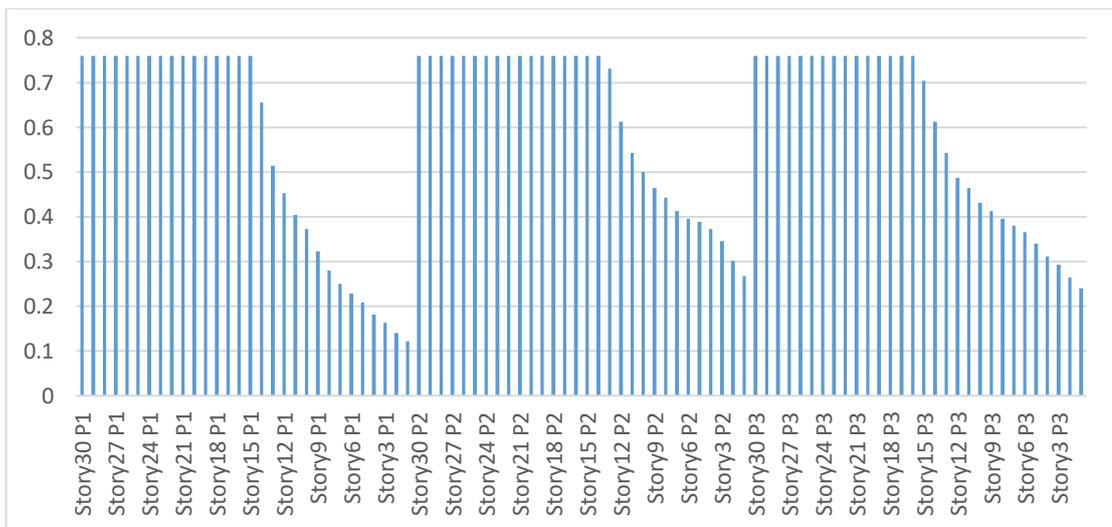
**Figure 4.31** Shear walls P-M-M D/C ratios.
