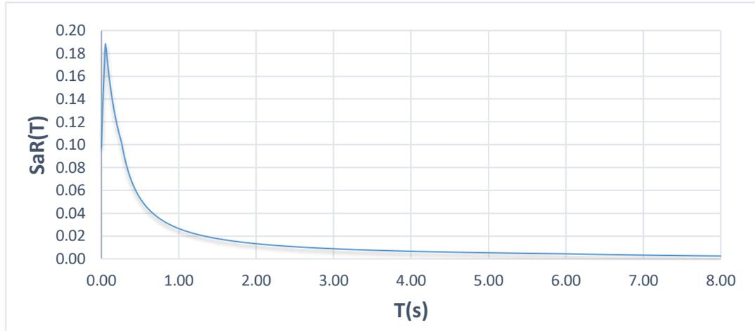
**Figure 4.8** DD-2 earthquake level reduced horizontal elastic design acceleration spectrum.
