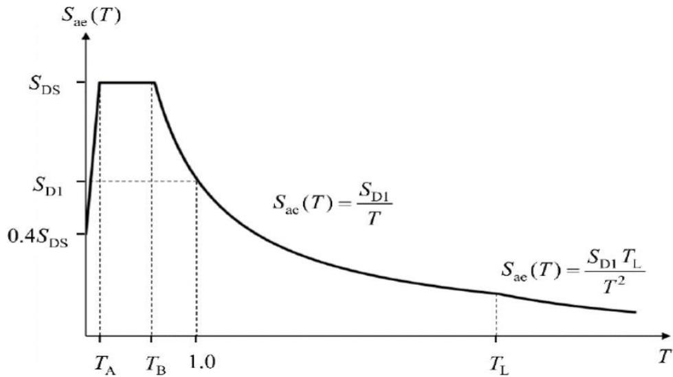
**Figure 3.2** Elastic design spectrum curve is given in TBDY 2018.
