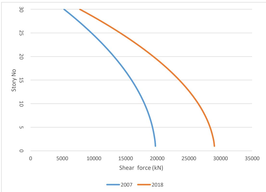
**Figure 4.47** Y direction story shear forces
