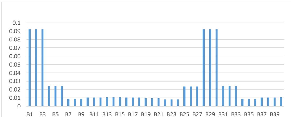
**Figure 4.24** Shear force D/C ratios of 20th floor beams.
