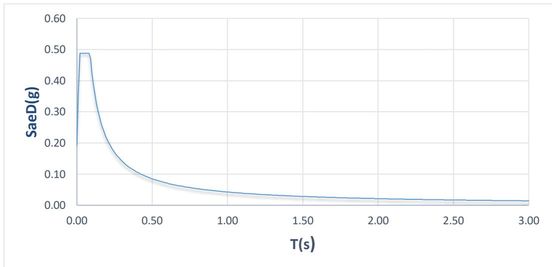
**Figure 4.7** DD-2 earthquake level vertical elastic design acceleration spectrum.
