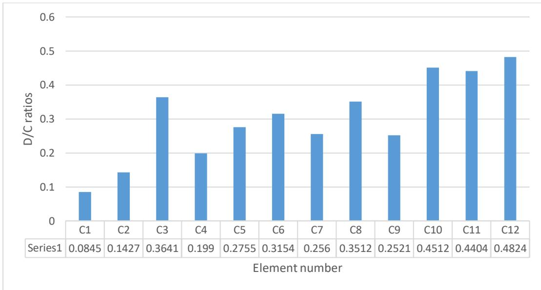
**Figure 4.39** 30th floor column P-M-M D/C ratios.
