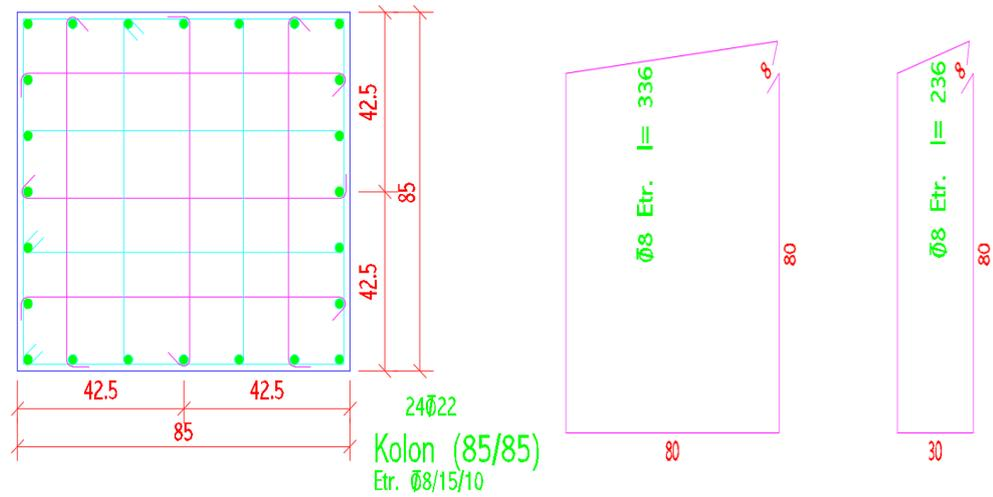
**Figure 4.16** 85 cm x 85 cm Column Reinforcements and Stirrups.
