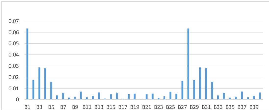
**Figure 4.28** Moment D/C ratios of 20<sup>th</sup> story beams.
