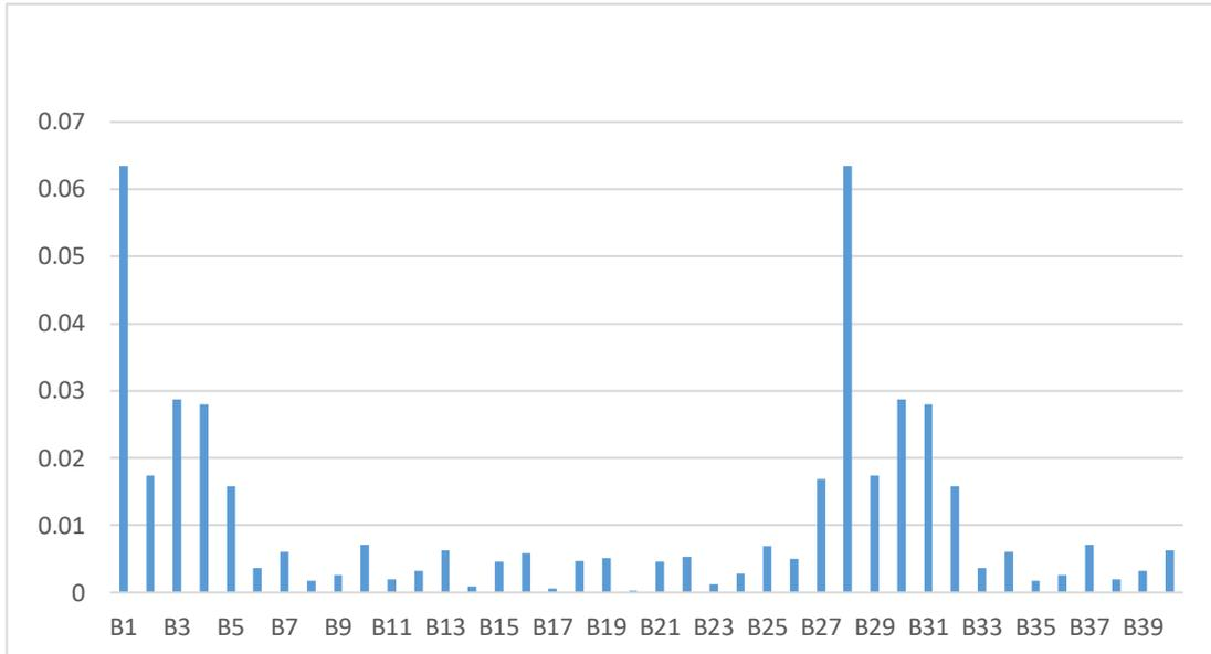
**Figure 4.29** Moment D/C ratios of 30<sup>th</sup> story beams
