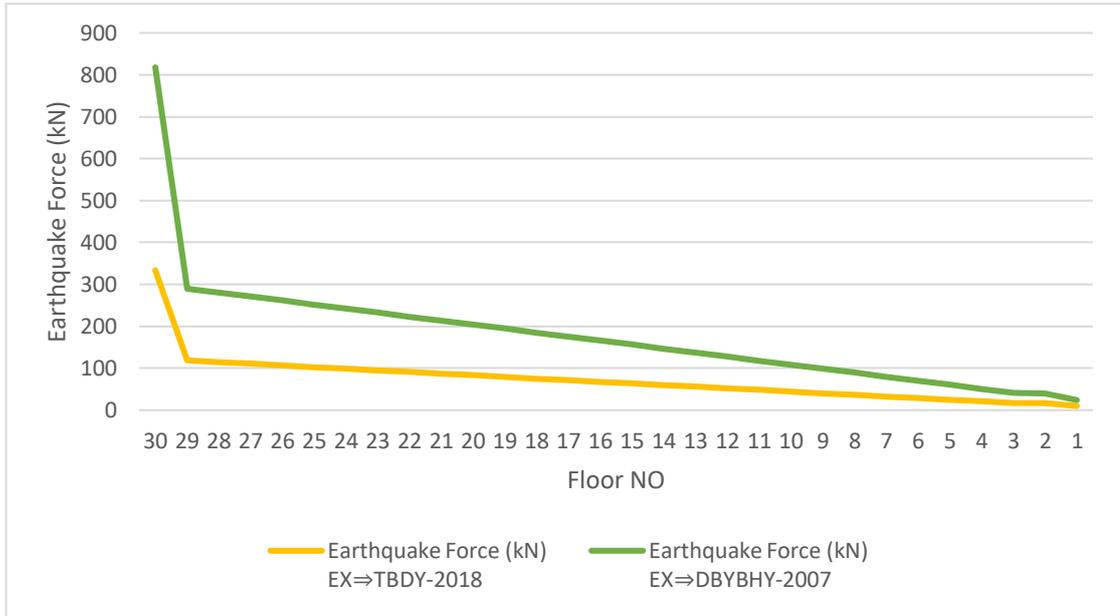
**Figure 4.40** Comparison of 2007 and 2018 X-Directional Seismic Forces.
