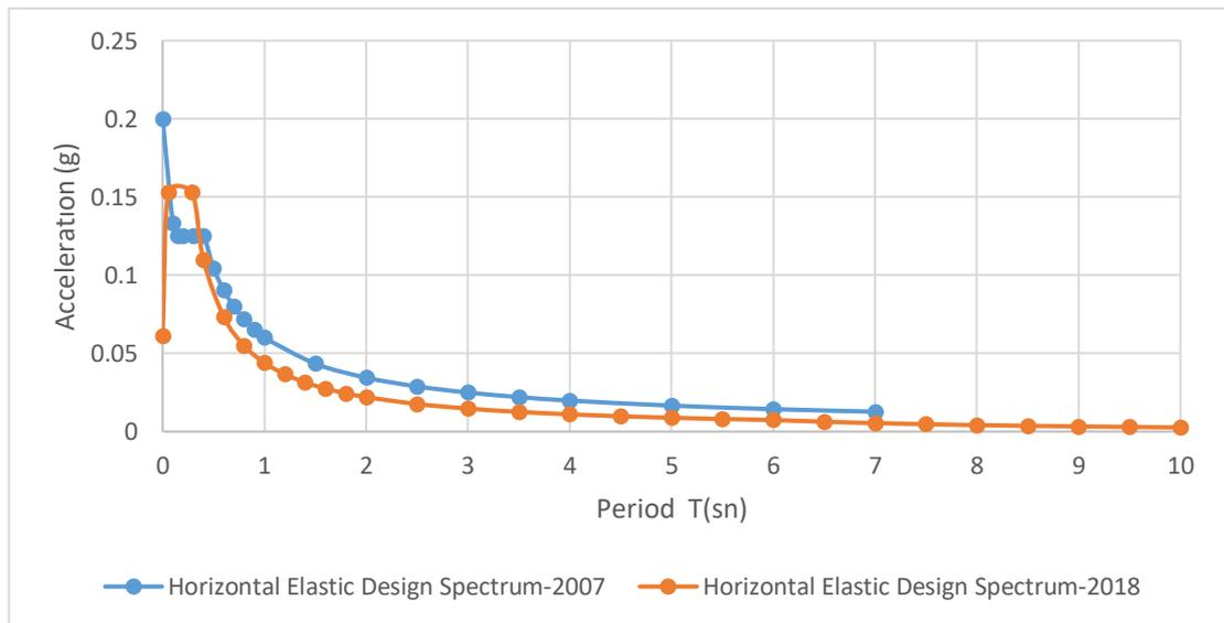
**Figure 4.42** Horizontal elastic spectrum comparison.
