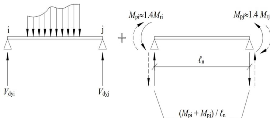
**Figure 3.8** Design shear force in beams (Celep, 2017).
