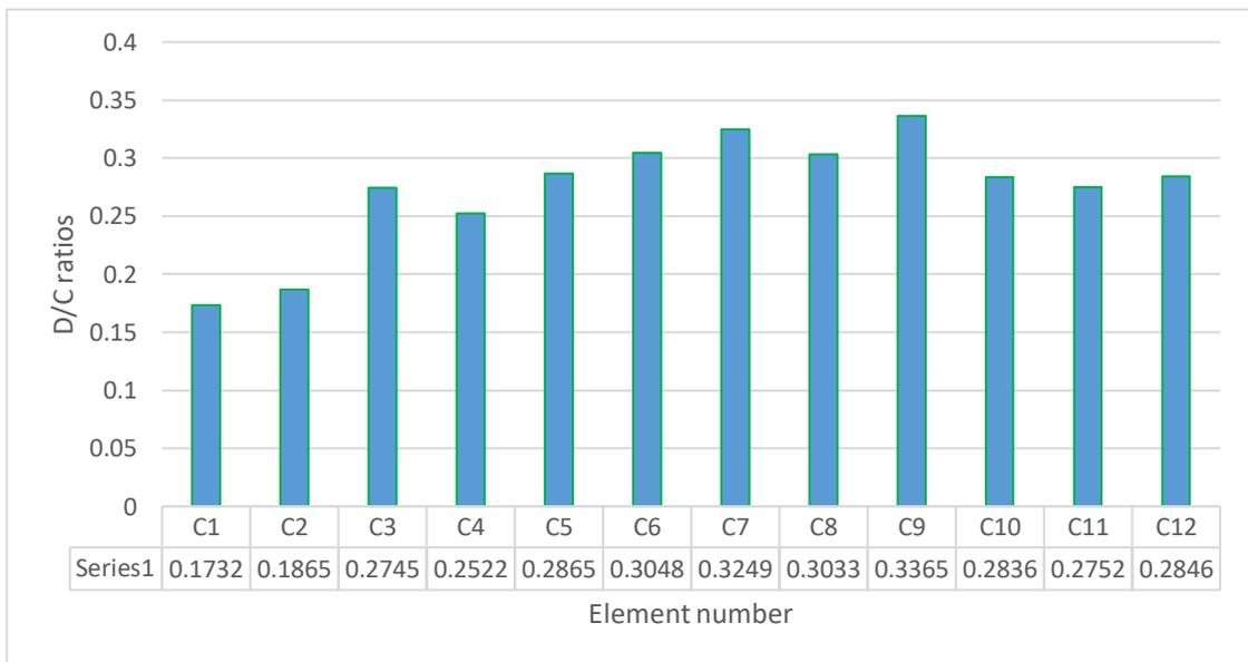
**Figure 4.37** 11th floor column P-M-M D/C ratios.
