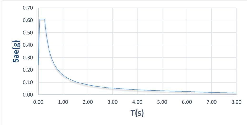
**Figure 4.6** DD-2 earthquake level horizontal elastic design acceleration spectrum.
