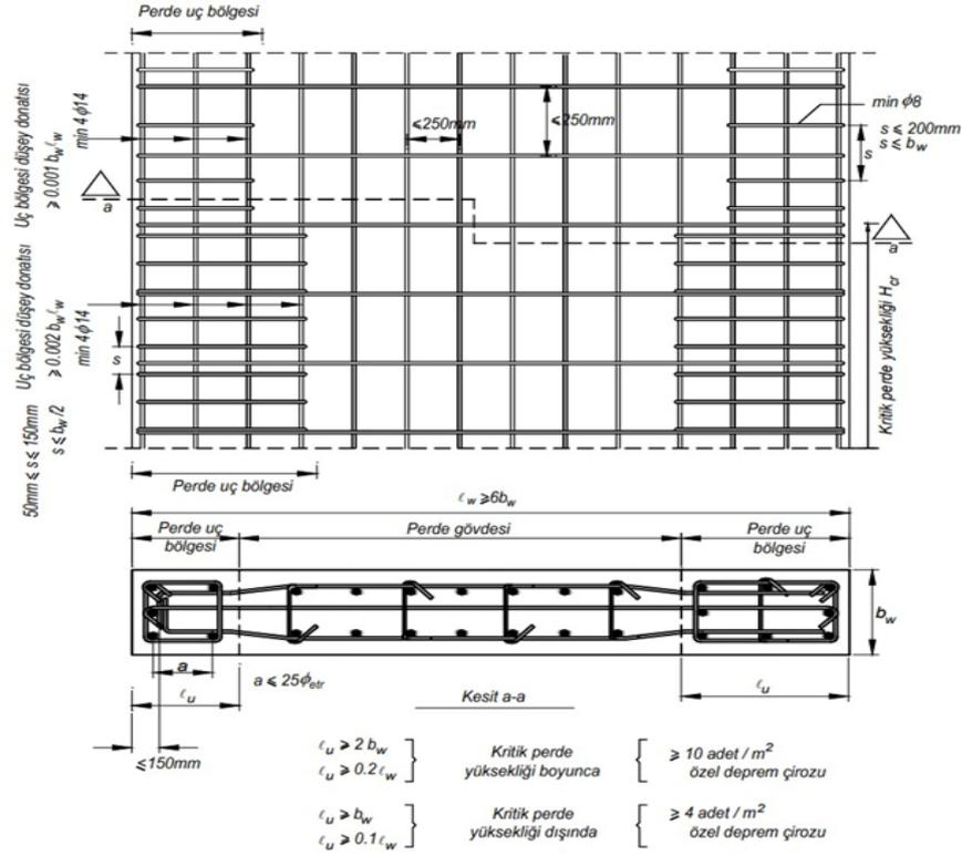
**Figure 3.10** Shear walls body and end reinforcements (Celep, 2017).
