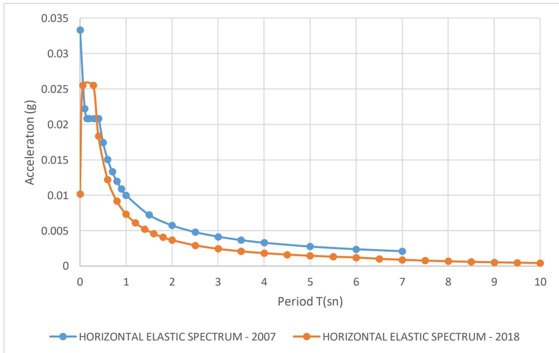
**Figure 4.43** Reduced horizontal elastic spectrum comparison
