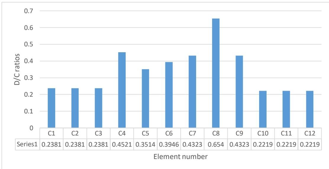
**Figure 4.35** 30th floor column shear force D/C ratios.
