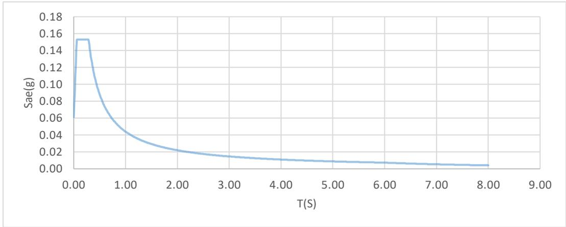
**Figure 4.17** DD-4 earthquake level horizontal elastic design acceleration spectrum.
