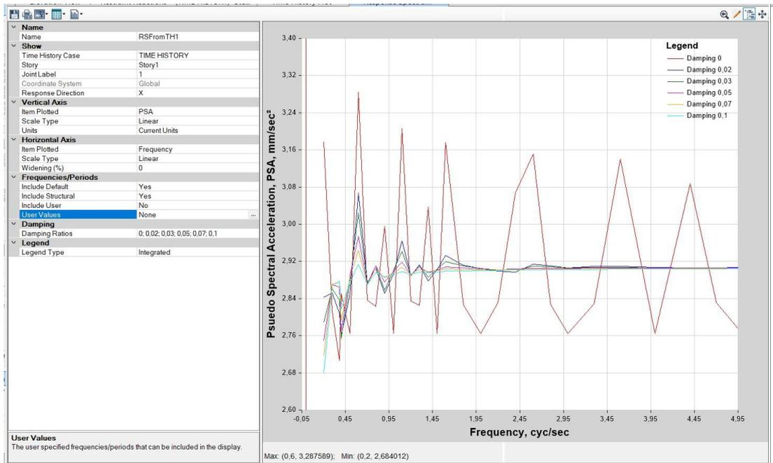
Figure 4.51 Scaled earthquake records.
