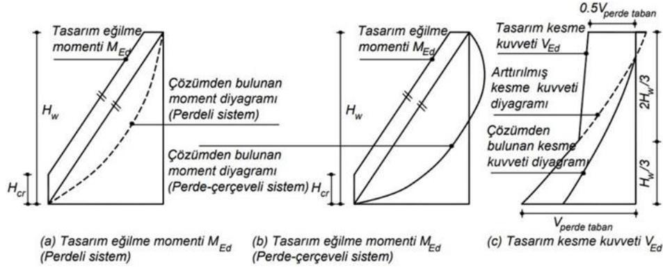
**Figure 3.9** Shear wall design Flexure moments (Celep, 2017).
