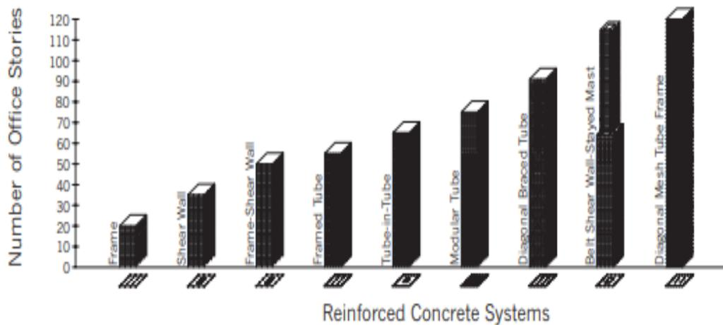
**Figure 3.1** Structural systems based on the number of stories (Sarkisian, 2016).
