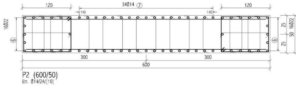
**c) Reinforcements of shear walls in 50 cm X 1300 cm Dimensions**
