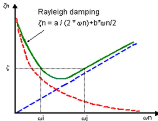
**Figure 3.11** Rayleigh damping function(Akçora, 2020).
