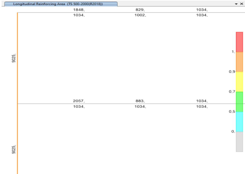
**Figure 4.14** Reinforcement area of columns from the Sap2000 program
