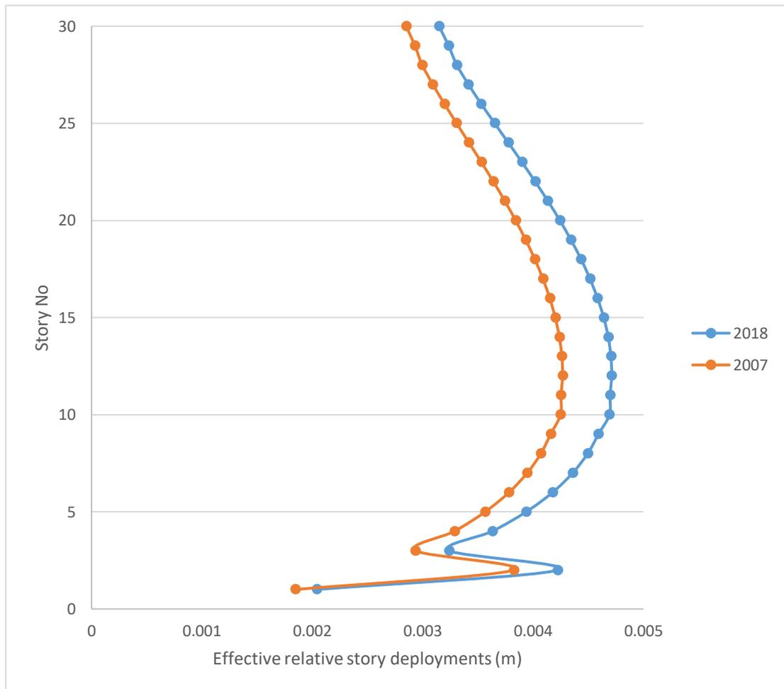
**Figure 4.44** Comparison of X-direction-enabled relative story offsets.
