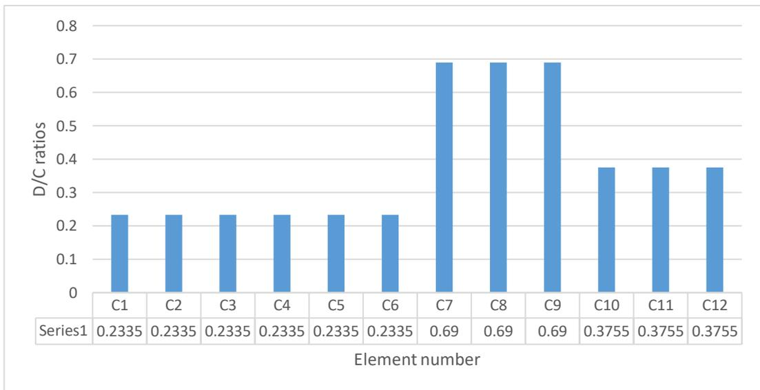
**Figure 4.32** 1st floor column shear force D/C ratios.
