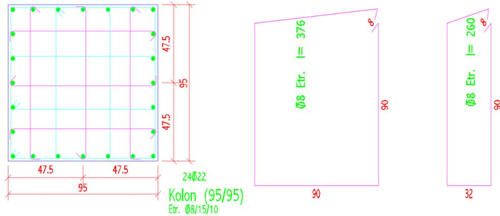
**Figure 4.15** 95 cm x 95 cm Column Reinforcements and Stirrups.
