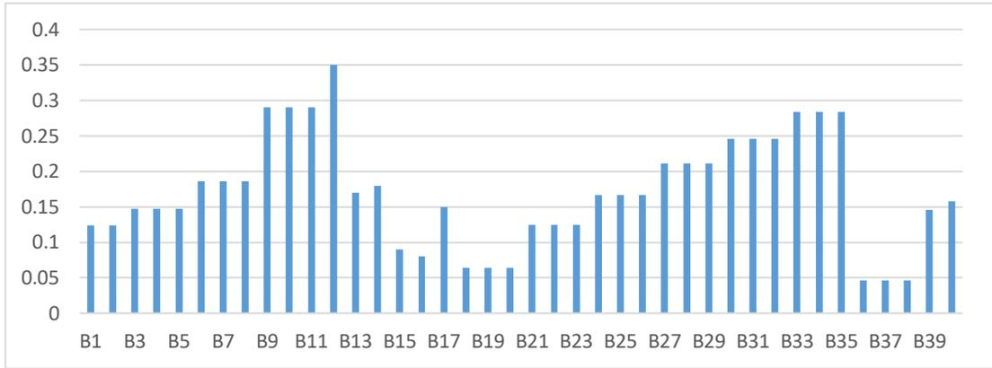
**Figure 4.22** Shear force D/C ratios of 1st floor beams.
