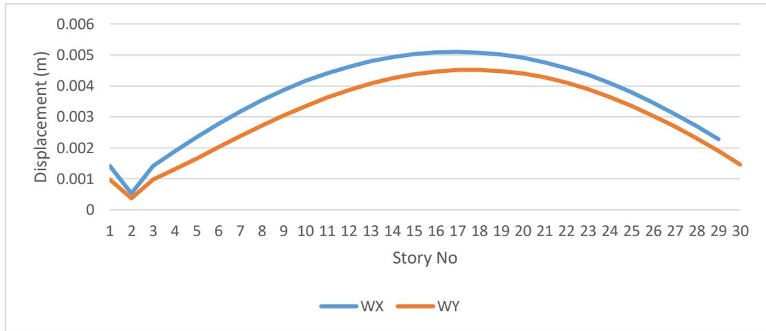
**Figure 4.5** Wind calculation maximum floor displacements
