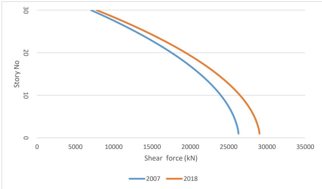
**Figure 4.46** Comparison of X-direction story shear forces.
