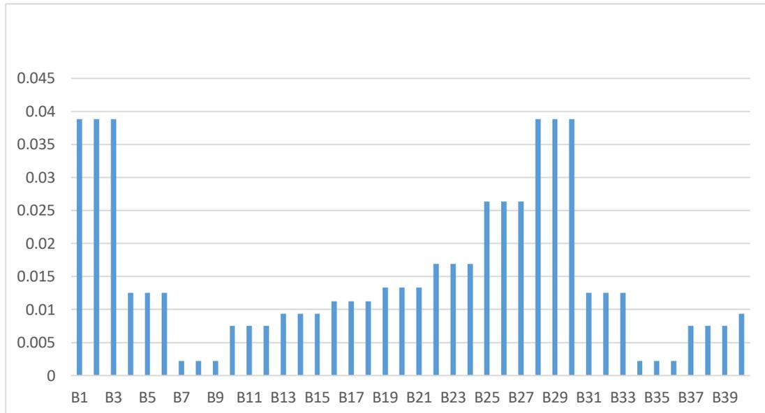
**Figure 4.25** Shear force D/C ratios of 30th floor beams.
