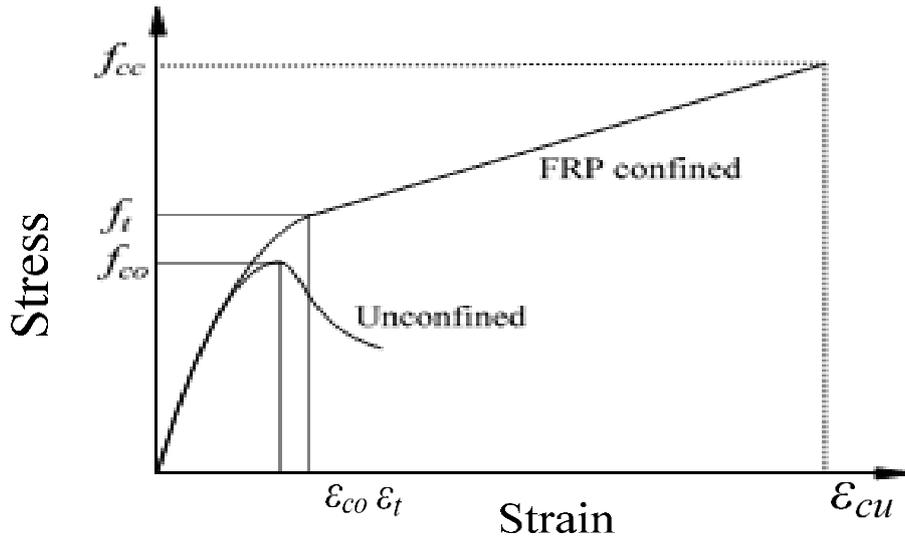
**Figure 3.5** The typical stress-strain curve for FRP-confined concrete with strain hardening. (Cao, Y. G., Jiang, C., & Wu, Y. F. (2016)).
