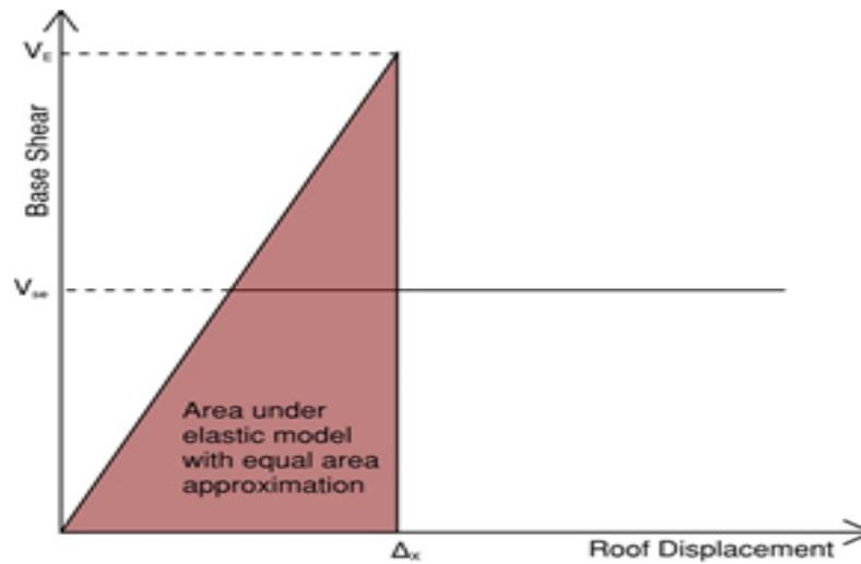
**Figure 3.3** Push-over curve of elastic-perfectly plastic EPP.
