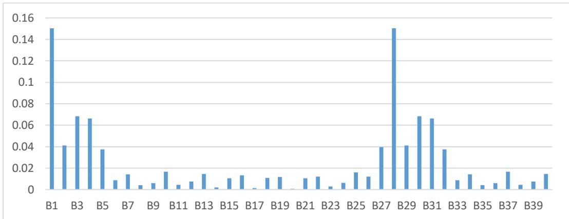
**Figure 4.27** Moment D/C ratios of 11<sup>th</sup> story beams.
