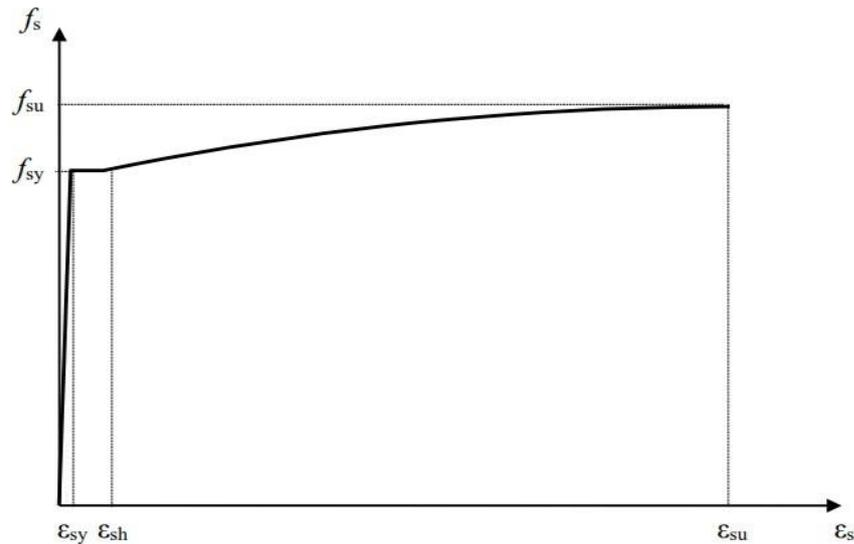
**Figure 3.6** Stress-strain diagram of reinforced steel. (Celep, Z. (2017))
