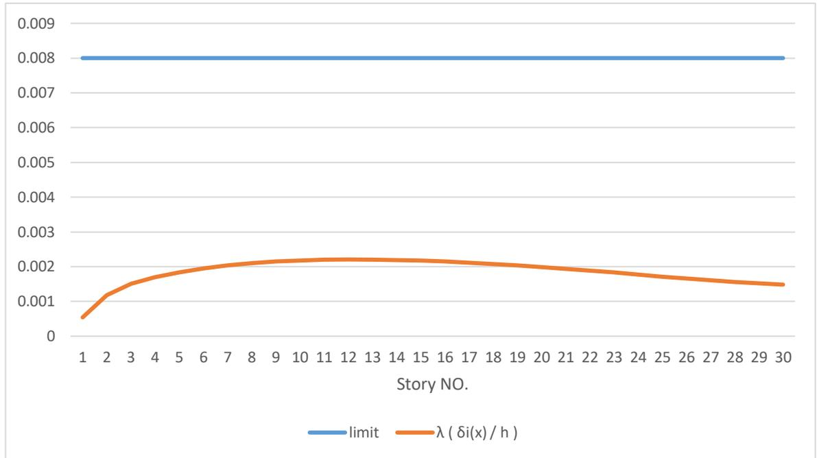
**Figure 4.10** The relative story drifts in X-X directions.
