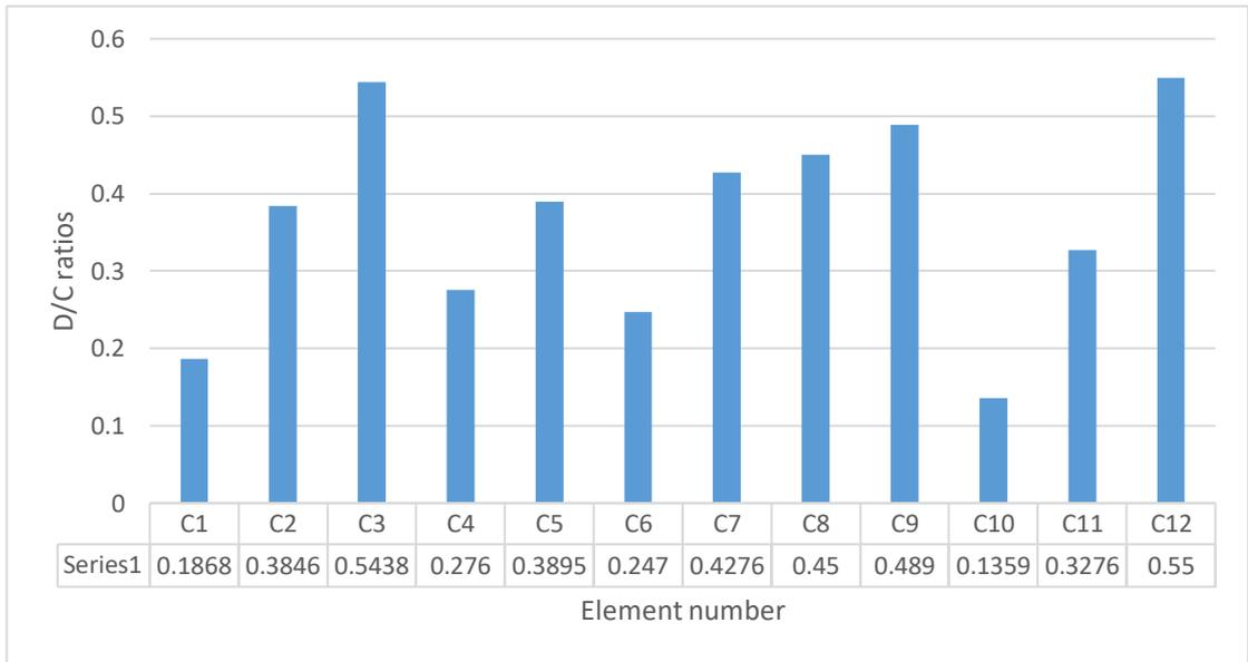
**Figure 4.36** 1st floor column P-M-M D/C ratios
