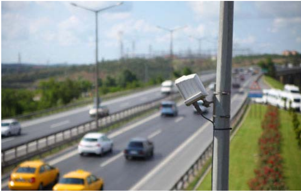
Figure 4.1 Traffic Sensor mounted on pole
